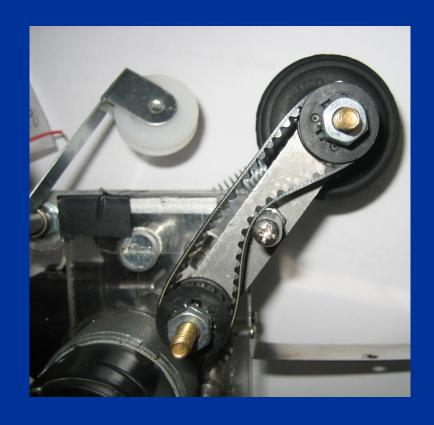
In this way one motor moves two wheels, one clockwise and one contraclockwise
