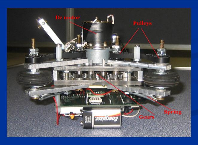
The motor transmit the torque to the wheeled arms through a pinion gear and then to the wheels by a transmission belt
