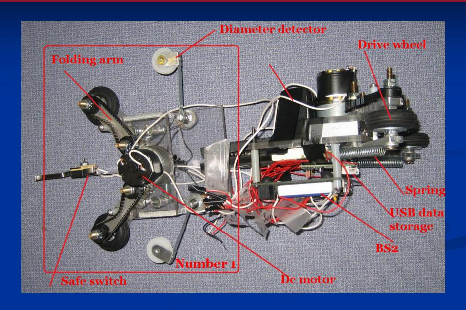
Since weight is a critical parameter, materials used have to be light and easily machinable: plexiglass, aluminun, plastic.
