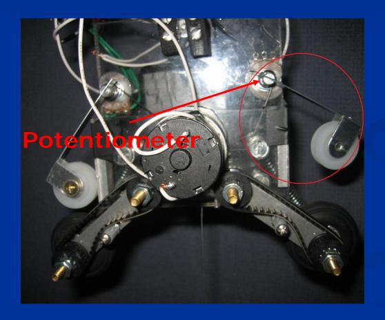
Angular displacement of the potentiometer is related to a variation of nominal diameter of the pipe and can be related to the presence of limestone
